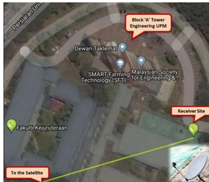
Figure 4. Aerial view of the experimental site, the ground station located in a futsal court with a clear canopy.
