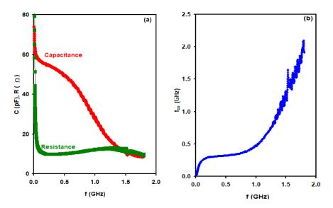
Fig. 3. (a) the resistance and capacitance spectra and (b) the microwave cutoff frequency spectra for Yb/WO<sub>2</sub>/Yb devices.
