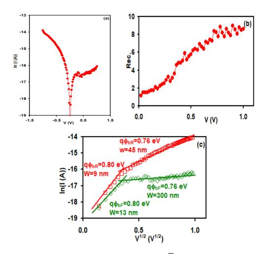
Fig. 2 (a) the ln(I) - V, (b) rectification ratio and the  $ln(I) - \sqrt{V}$  variation for the Yb/WO<sub>3</sub>/Yb diodes.
