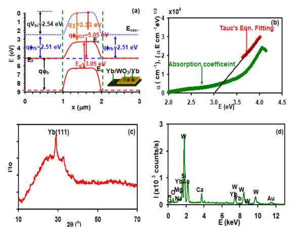
Fig. 1. (a) the energy band diagram, (b) the optical absorption and Tauc's equation fittings, (c) the X-ray diffraction patterns and (d) the energy dispersive X-ray spectra for  $Yb/WO_3/Yb$  films. The inset of (a) shows the schematics of the device.
