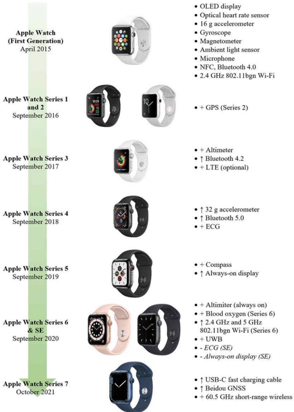
Figure 2: The development of Apple Watch Series functions. Upgrades to features (↑) and additions of new features (+) are mentioned. GNSS: global navigation satellite system; ECG: electrocardiogram; LTE: Long-Term Evolution; NFC: near-field communication; OLED [53].
