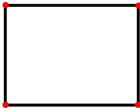
Fig. 2.2: A simple rectangular element with four nodes
