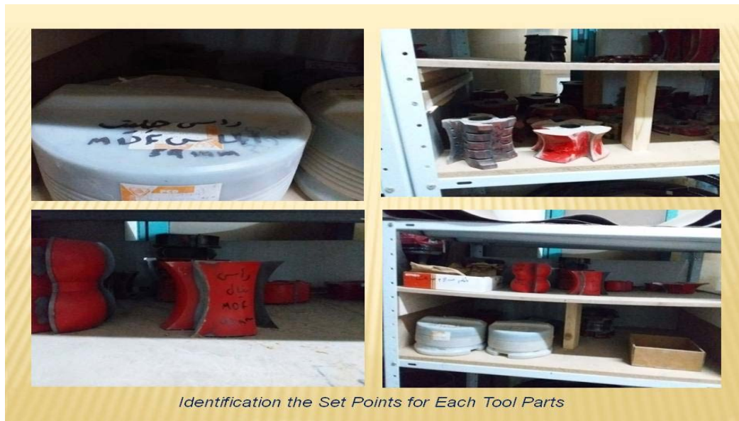
Figure 4-7: Identification of the Set Points for Each Tool Part by Using Black Marker
