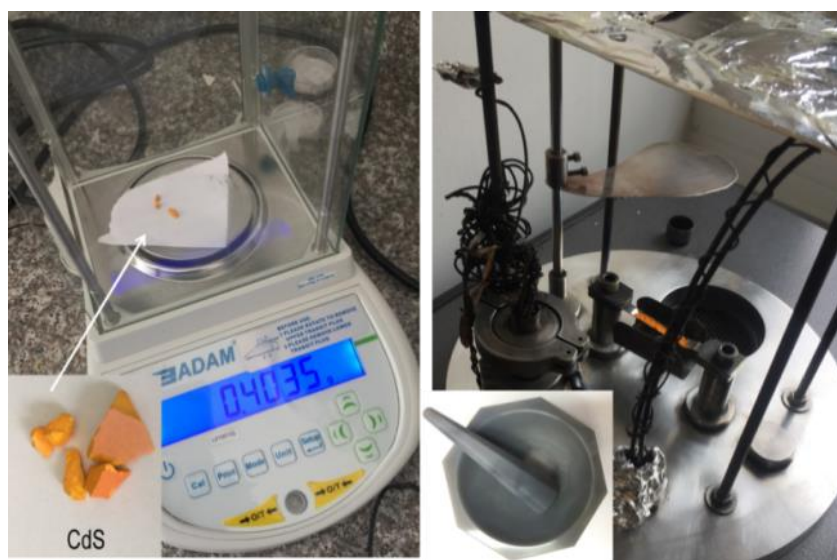
Figure 3.3. The setup of the evaporation process for the third and fourth runs.
