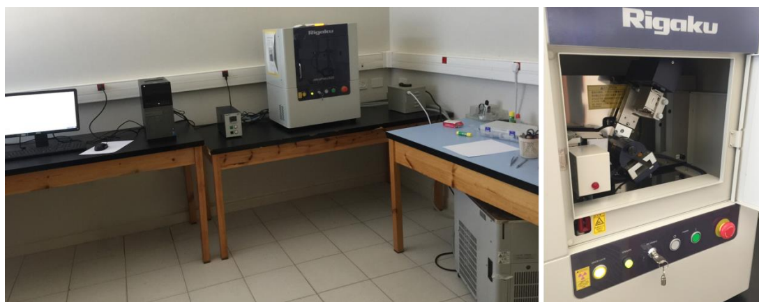
Figure 3.8: Rigaku MiniFlex 600 X-ray diffractometer.
