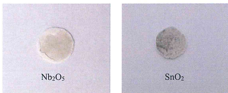
Fig 3.4. The optical image for \text{Nb}_2\text{O}_5 and \text{SnO}_2 powders after being compressed at 200 bar by a hydraulic press.
