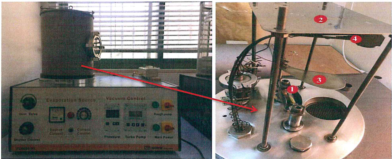
Fig 3.8. The VCM 600 thermal vacuum evaporation system. Item one is the tungsten boat, item two is substrate holder, item three is the metal plate, and item four is the high-resolution INFICON STM-2 thickness monitor.
