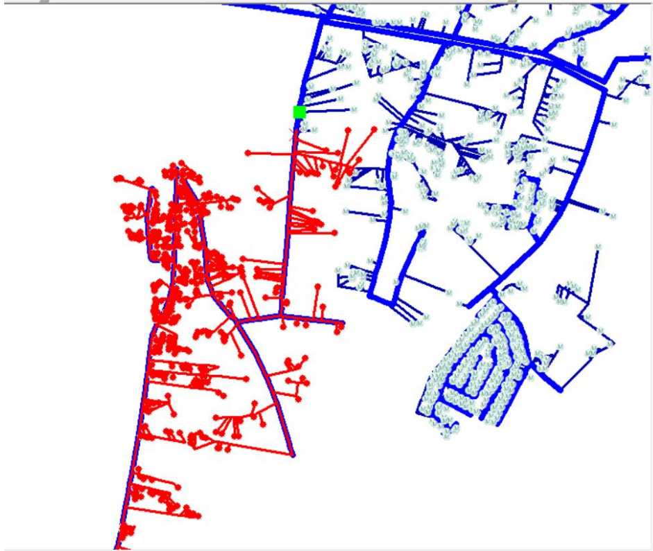
Figure 22: The Geometric Network Connected and Disconnected using the Utility Network Analyst toolbar.
