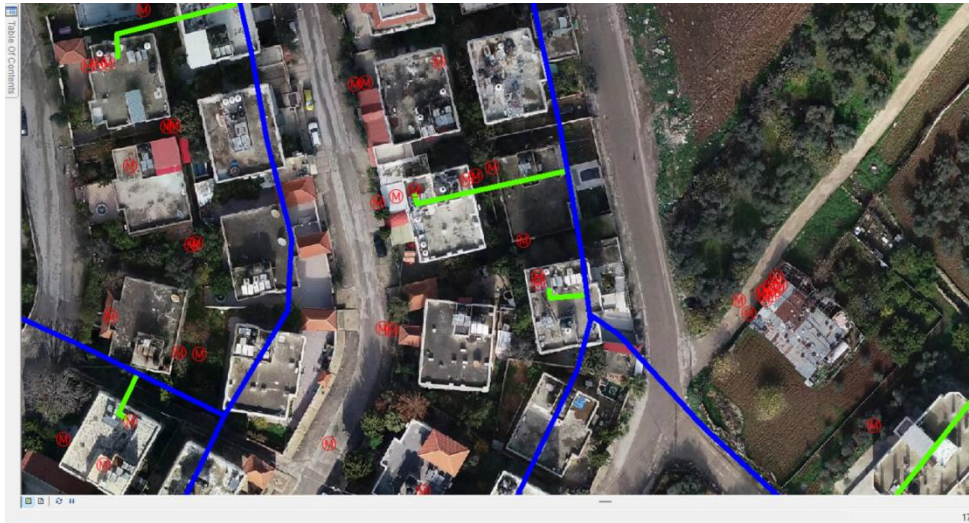
Figure 10: (a) Meters without connections to main pipe. (b) The map with the aerial image.
