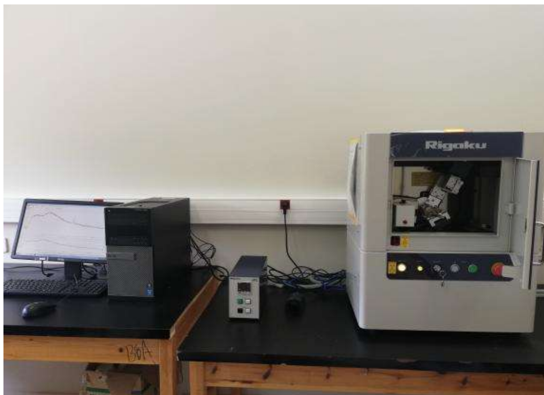
Figure 3.2: The Rikago Miniflex 600 diffractometer.
