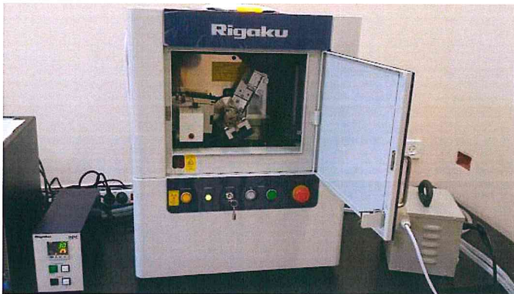
Fig. 3.2: Rikagu Miniflex 600 diffractometer.
