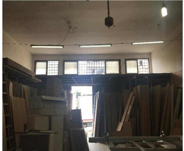
Figure 18 Implementing 5S in Storage Loft C which has then been emptied and then ready to be dismantled and reassembled next to Loft B
