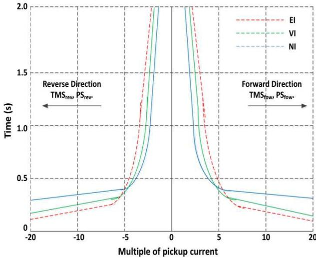
Fig. 1. Time-current characteristics for dual-setting DOCR [8].
