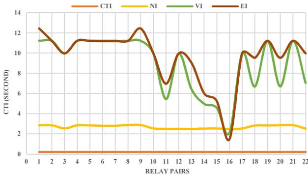
Fig. 4. CTI values of dual-setting DOCRs for different relay standard characteristics in islanded mode.
