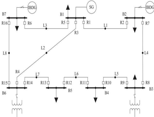
Fig. 2. Single line digaram of the 7-bus AC microgrid system [3].
