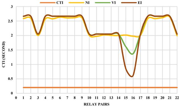
Fig. 3. CTI values of dual-setting DOCRs for different relay standard characteristics in grid-connected mode.
