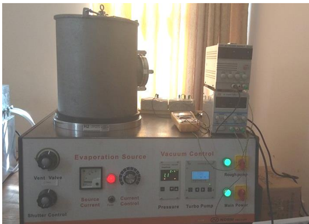
Fig. 3.1. The 600 VCM evaporation system.
