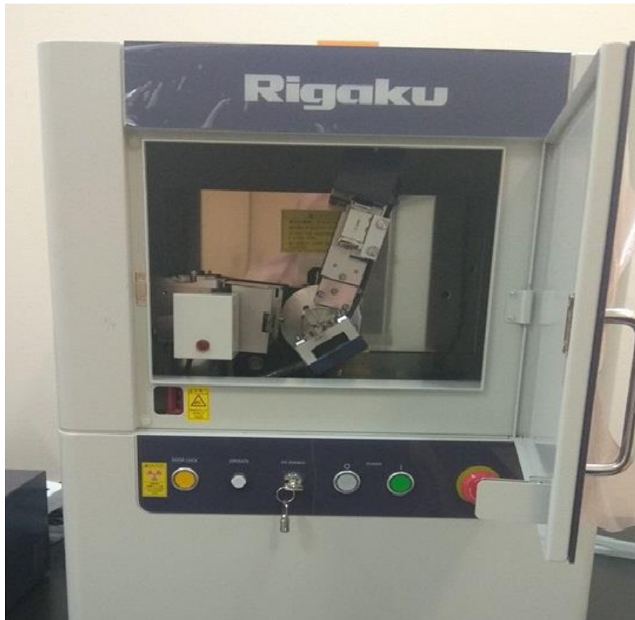
Fig. 3.5. Rigaku diffractometer for the 1.542\text{\AA} Cu XRD.
