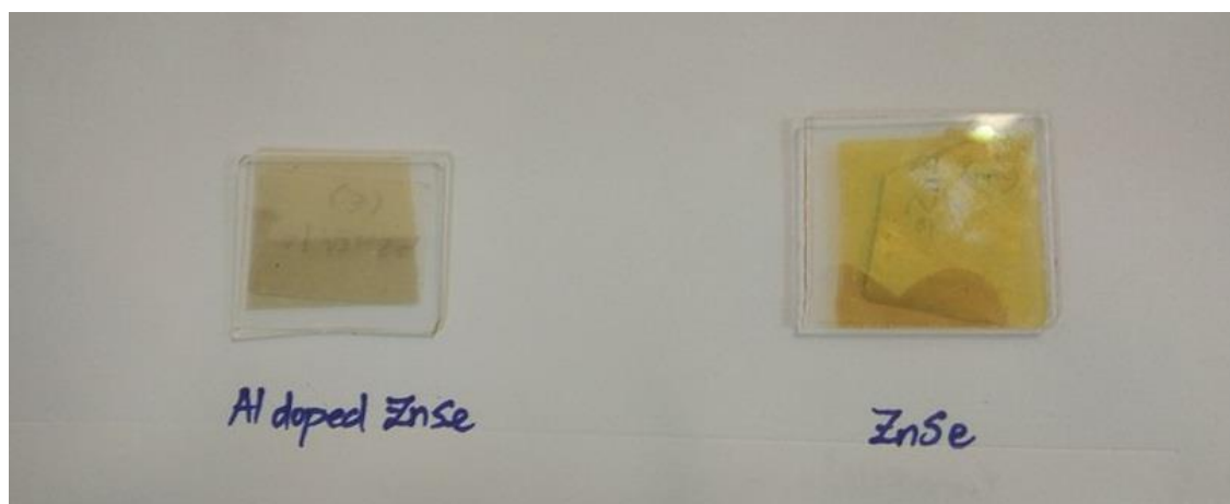
Fig. 3.2. The ZnSe and Al doped ZnSe thin films grown on a glass substrate.
