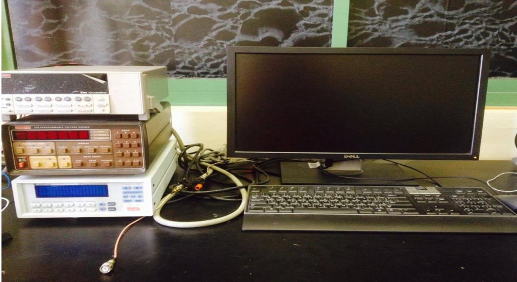
Figure 3.11: Current-voltage (I-V) measurement including Keithley 6485 Picoammeter and Keithley 230 Voltage Source.
