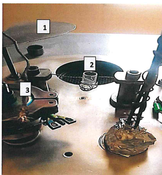
Fig 3.1: The illustration of the quartz boat in the evaporation source (item 1 for Shutter ,item 2 for quartz boat , item 3 for thermocouple ) .
