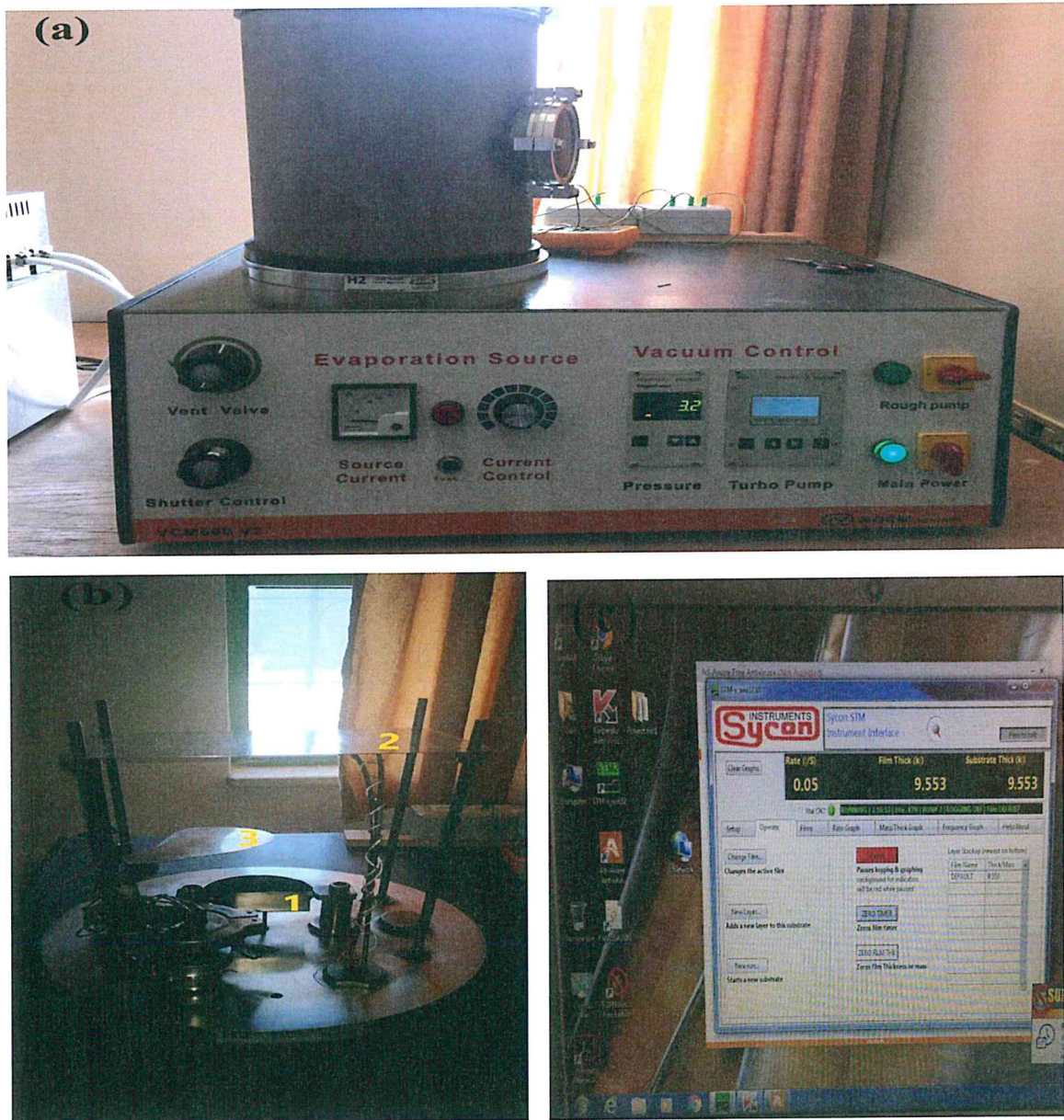
Figure 3.3: (a) The VCM-600 thermal evaporator (b) the inside of VCM-600 and (c) the screen of the thickness monitor.
