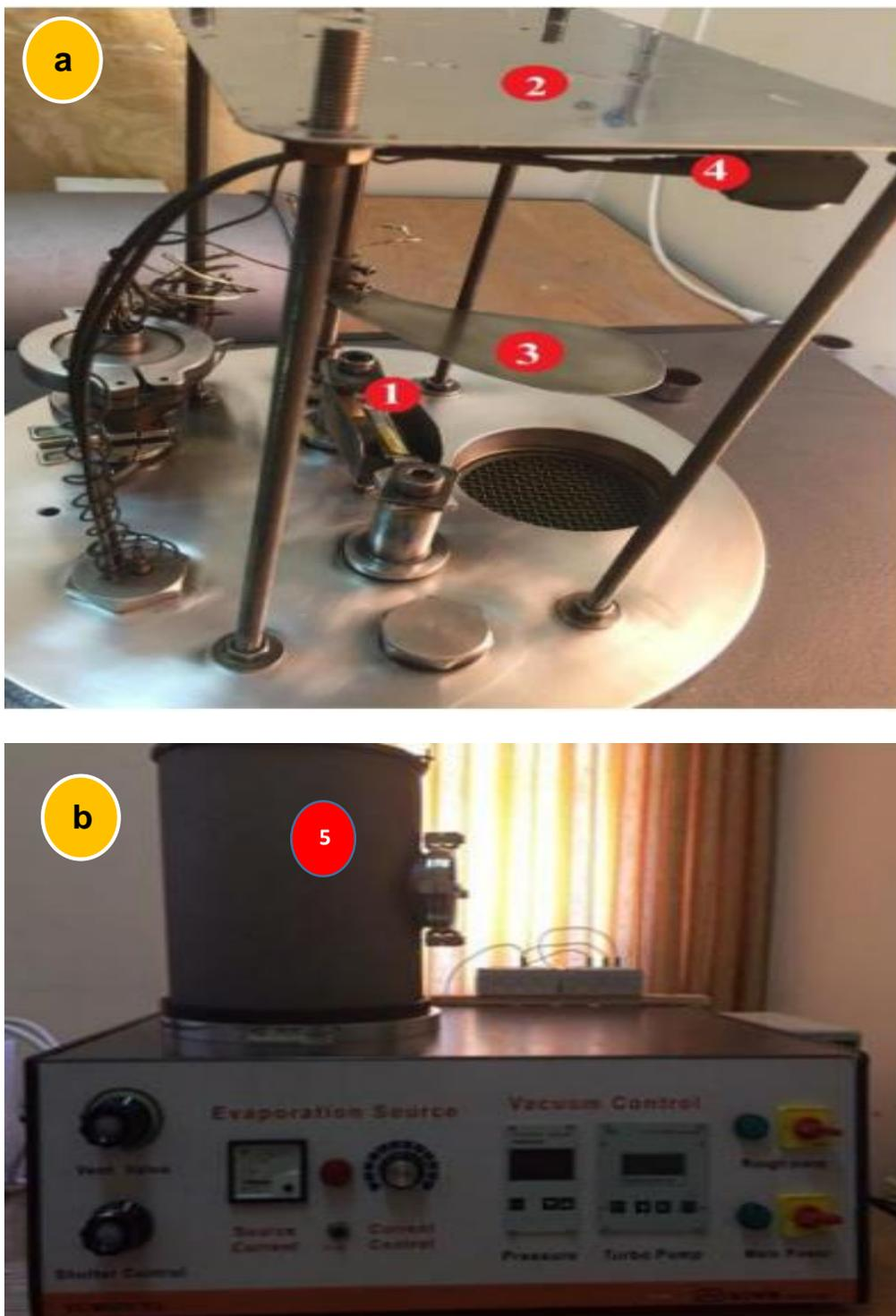
Figure 3.1: The physical vapor deposition system. a. from inside. b. from outside.
