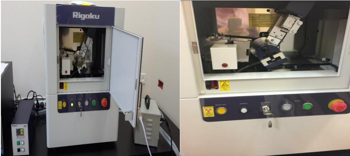
Figure. 3.5: Rigaku Miniflex 600 diffractometer.
