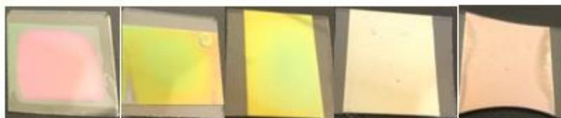
Figure. 3.3 optical image nanosandwiched films  $d=0, 50, 75, 100$  and  $200\text{nm}$ .
