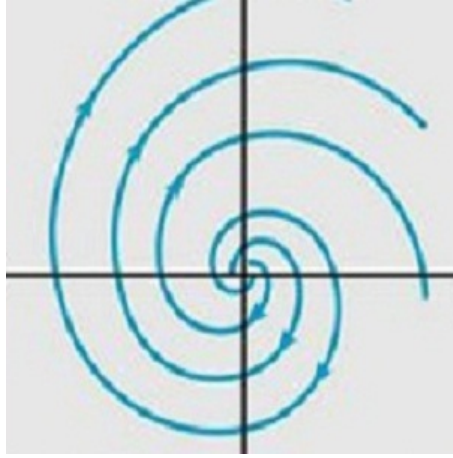
Fig. 3.1: Stable limit cycle
