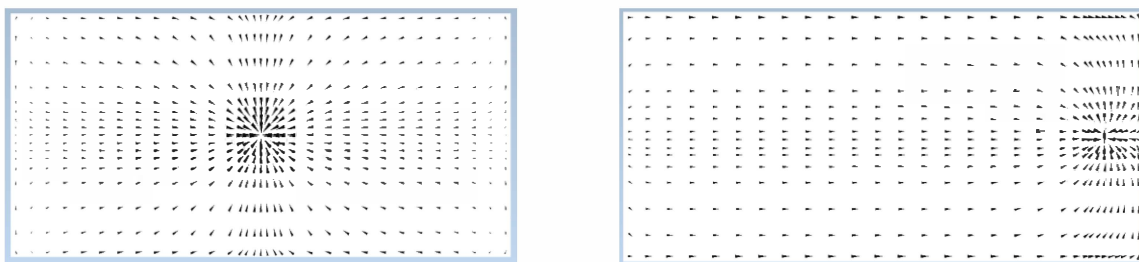
Fig.4: Current distribution for MP at the center (2.45 GHz) and at middle of the short edge of the chassis (1.2 GHz).
