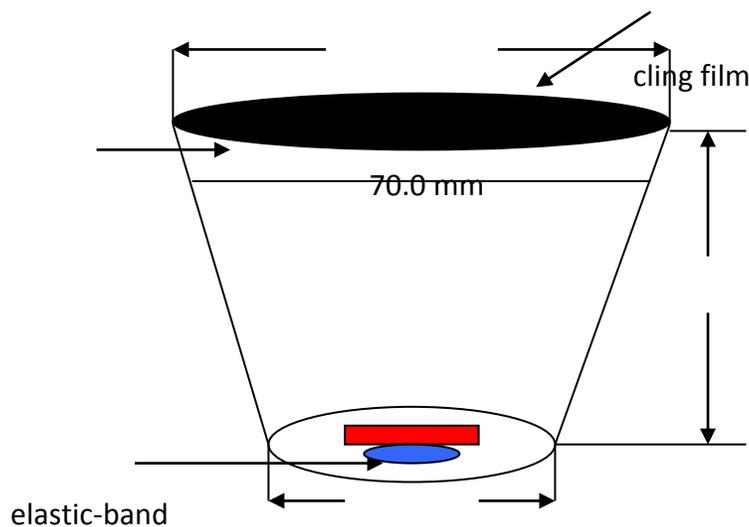
Figure 2. Typical CR-39 Dosimeter
