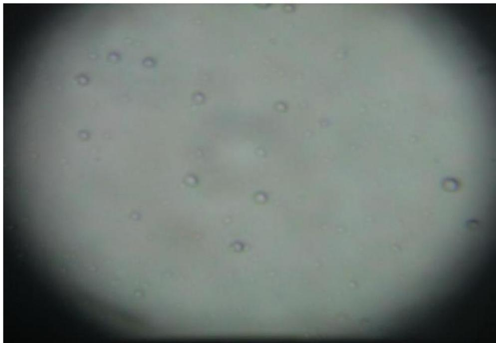
**Figure 4. Tracks of Alpha Particles Emitted by Radon in a CR-39 Detector Magnified 200 Times, which was Exposed for Six Months in the Third Floor of Engineering Building.**
