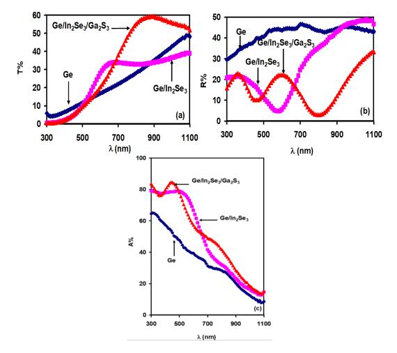
Fig. 2. (a) The transmission coefficient, (b) the reflection coefficient and (c) the absorbance spectra for the Ge,  $Ge/In_2Se_3$  and  $Ge/In_2Se_3/Ga_2S_3$  interfaces being recorded at room temperature.
