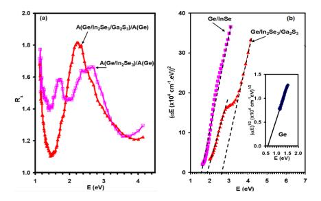
Fig. 3. (a) the absorbability spectra and (b) the Tauc equation plots for the  $Ge/In_2Se_3/Ga_2S_3$  interfaces.
