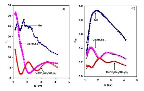
Fig. 4. (a) The real and (b) the imaginary parts of the dielectric spectra for the Ge, Ge/In<sub>2</sub>Se<sub>3</sub> and Ge/In<sub>2</sub>Se<sub>3</sub>/Ga<sub>2</sub>S<sub>3</sub> interfaces. The sold dark lines of (b) indicate the fittings obtained by Eqn. 1.
