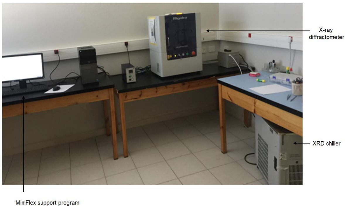
Figure 3.8. The Rigaku MiniFlex 600 X-ray diffractometer.
