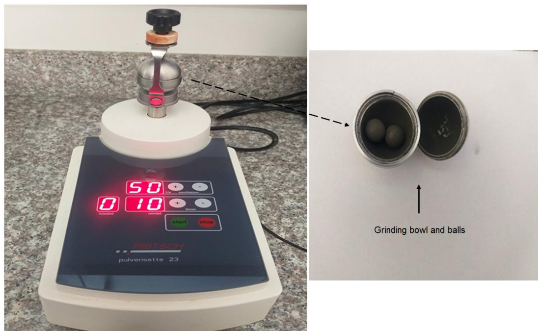
Figure 3.3. The Fritsch Pulverisette 23 mini mill grinder with grinding bowl and balls.
