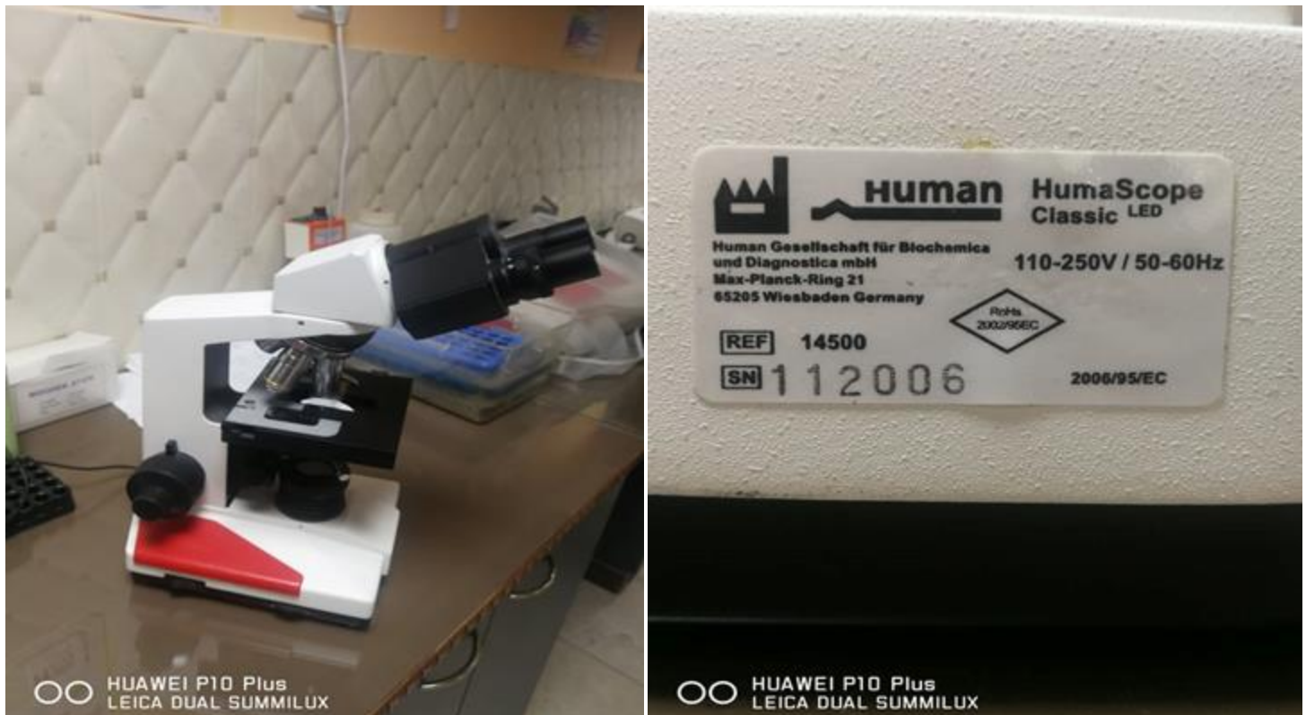
Figure 2.5 : Shows the microscope that was used in counting the traces of alpha particles , with some information as SN and REF
