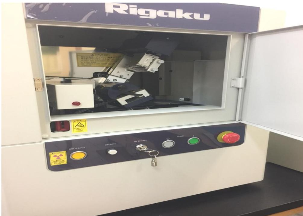
Figure 3.4: The X-ray diffraction technique (XRD)
