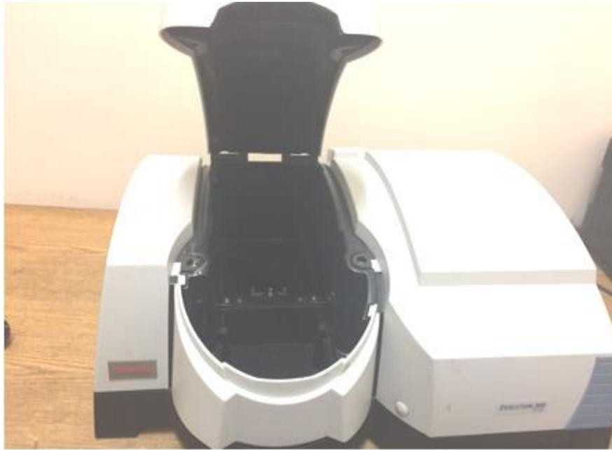
Figure 3.5: The UV-VIS spectrophotometer.
