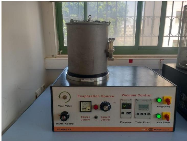
Fig. 3.2 The 600 VCM evaporation system.
