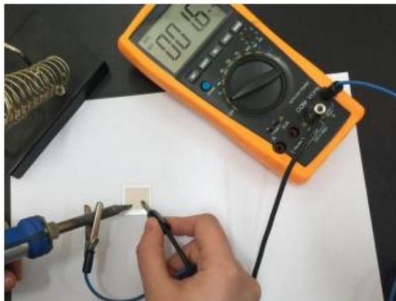
Fig. 3.5 The set-up of hot-probe technique.
