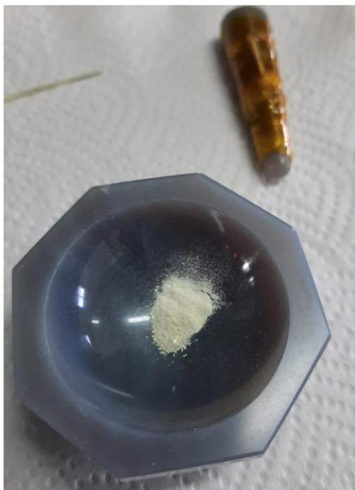
Figure 3.4: Mortar and pestle to crush ceramics pellets into fine powder.
