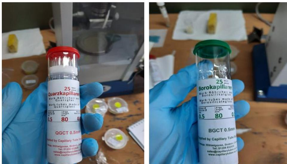
Figure 3.9: Quartzkapillaren (the red one) and borokapillaren (the green one).
