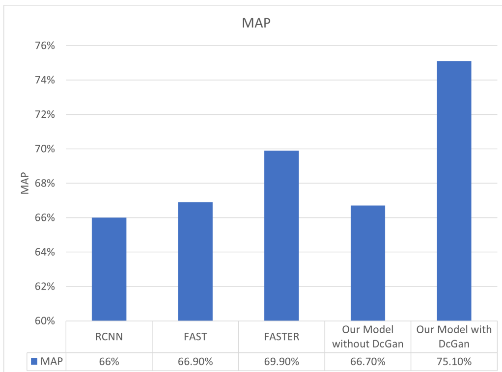
Figure 7. Comparison between RCNN, Fast R-CNN, Faster R-CNN, and the proposed model detection precision
