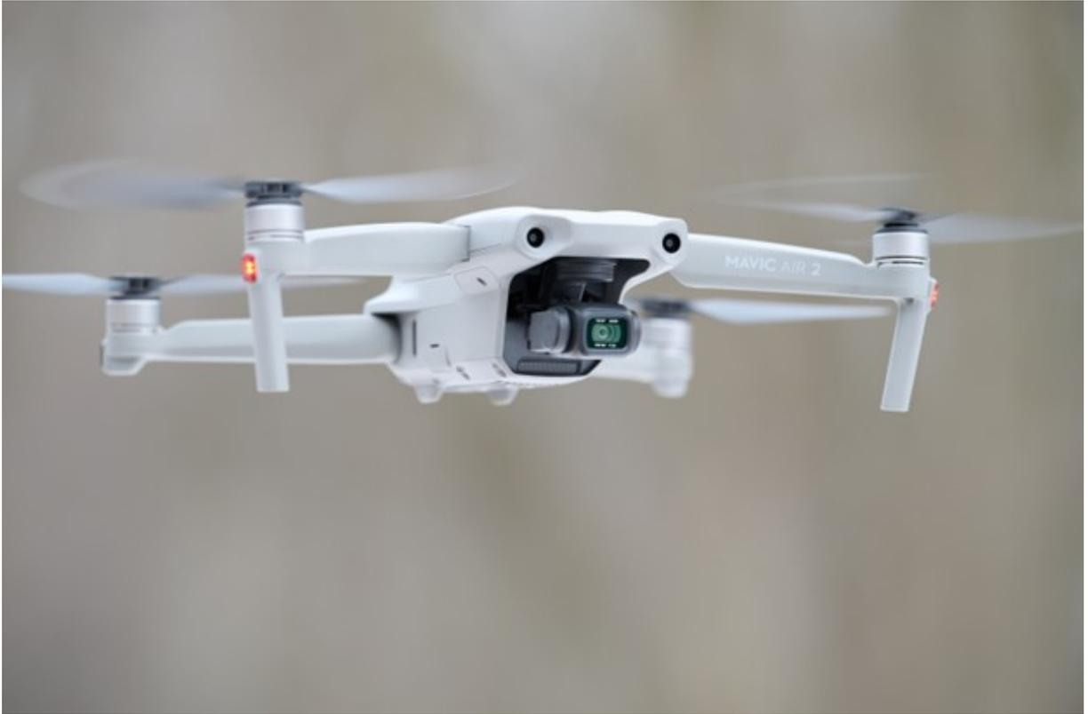
**Figure 3.2:** DJI Mavic Air 2 Drone
