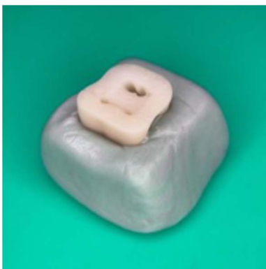
Fig 3. Photograph of a 3D-printed artificial tooth model fixed into a silicone block before irrigation.
