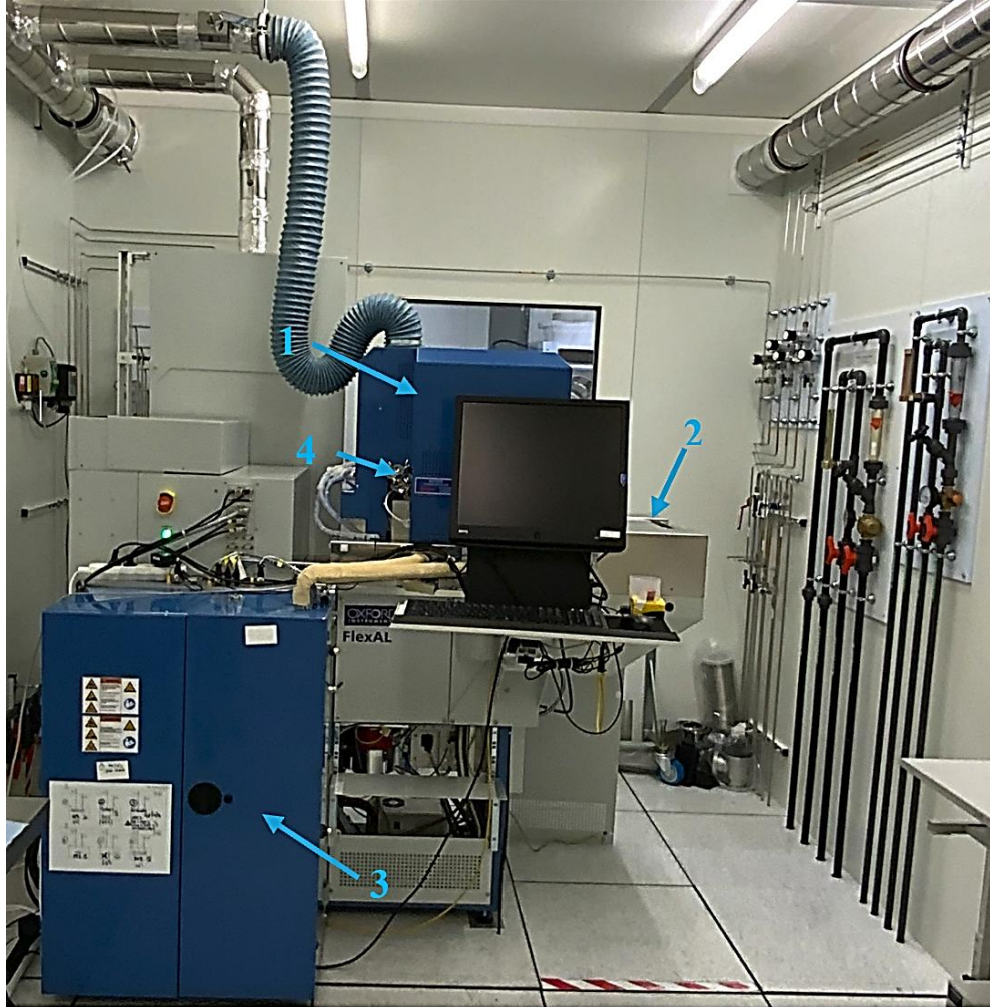
Figure 3.5: ALD Flexal reactor developed by Oxford equipment's Located at BCAI clean room in CIME.
