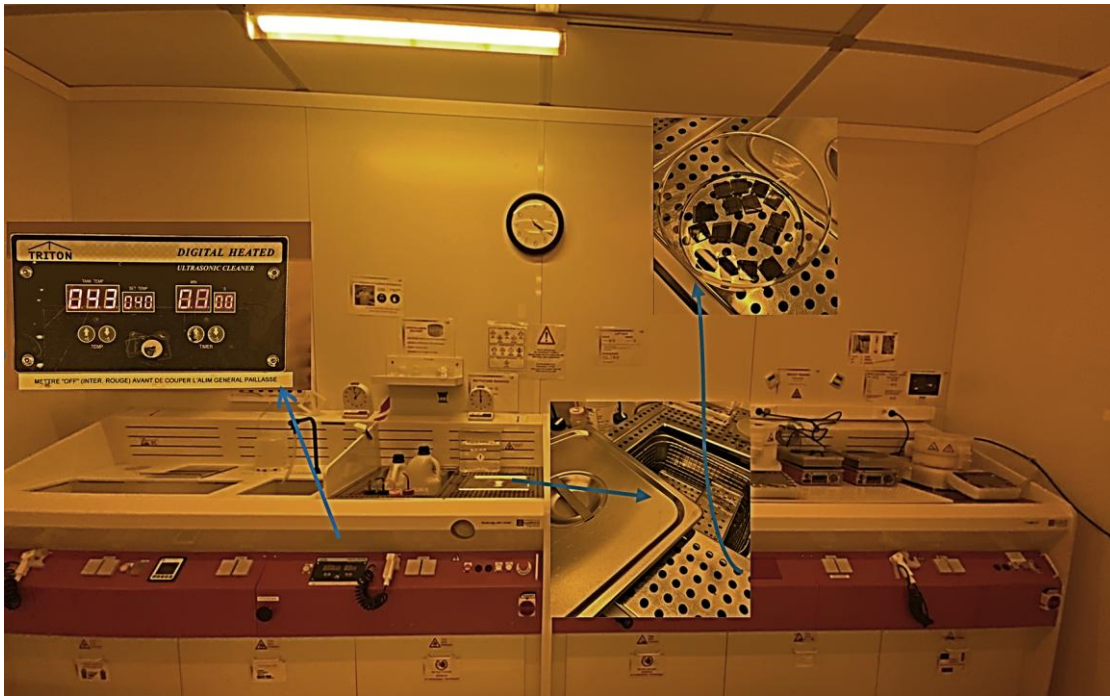
Figure 3.9: Chemical bench in BCAI clean room highlight samples prepared for stripping in US bath, US plate and setting screen for US cleaner.
