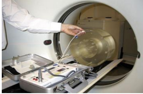
Figure 2.1: CTDI PMMA phantoms of standard size, with an axial length of 14 cm. diameters: 16 head and 32 cm body, with an electrometer and ion chamber measuring 100 mm (Edyvean et al., 2012).
